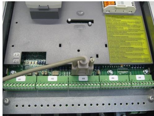
Connect the DCS550 via X34 to the PC COM port
