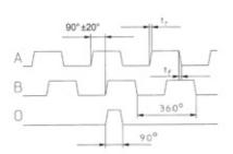
Using the sensor outputs of the encoder, the voltage
