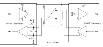
Encoders with internal termination have a fixed terminating resistor Rt built in.
