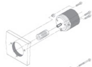
Mounting with assembly bell, fastening eccentrics and coupling (to prevent shaft overload and to isolate the encoder thermally and electrically).
