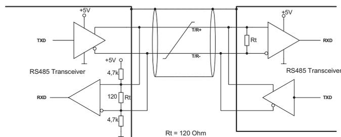
Encoders with internal termination have a fixed terminating resistor  $R_t$  built in.
