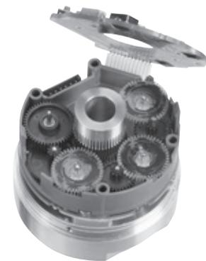
**The patented electronic electronic Sendix multiturn stage with Intelligent Scan Technology™**
