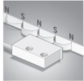
The distance between the sensor and the magnetic band can be up to 2 mm.
