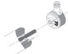
Mounting of a hollow shaft encoder with extended torque stop and long pin.
