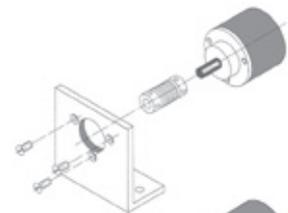
Mounting with a commonly used clamping device and coupling (to reduce shaft overload).
