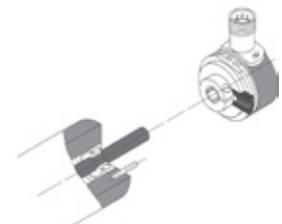
Mounting of a hollow shaft encoder with a stator coupling.
